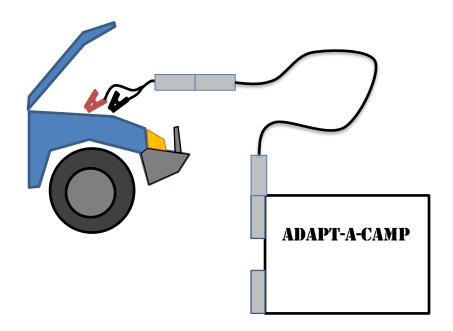
This set up is possible and usable, but care must be taken not to drain the vehicle battery to a point which it will not start your engine! Keep an eye on that voltmeter! There is no specific safe voltage reading, that we can specify as being able to still start your engine. There are many variables in this situation including
